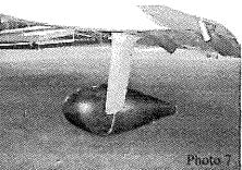
through the join line is that I was not able to cut through neatly on the upper side of the gear leg. After much application of dry micro and even more sanding, the pants are ready for painting. Following are some photos will be of the finished product.
