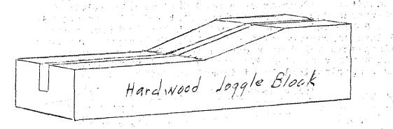
(2.) Another quickey to joggle 3/4" x 3/4" angle as in forward fuselage modification. Place angle, not too tightly in soft jawed vise, support horizontal flange with spacer slightly thicker than depth of joggle. Hold heavy block of steel on top of angle and hammer the unsupported end down.
