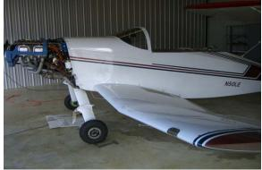
Aircraft partially disassembled for condition inspection
