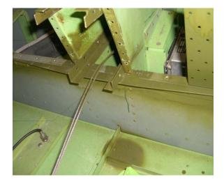
Aft looking forward- four  $\frac{3}{4} \times \frac{3}{4} \times \frac{1}{16}$  inch angles in tunnel 505 replaced due to corrosion. Forward end of baggage compartment tunnel is attached to these angles. Corrosion removed to ~ 20% depth in upper carry through spar cap at location of tunnel interface. A double tapered angle doubler was riveted to the aft side to maintain structural integrity.
