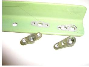
Note steel anchor nut plates were attached before primer applied.
