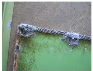
Bottom side of tunnel top piece that attached to side panel shown above. Note carpet glued to top surface.
